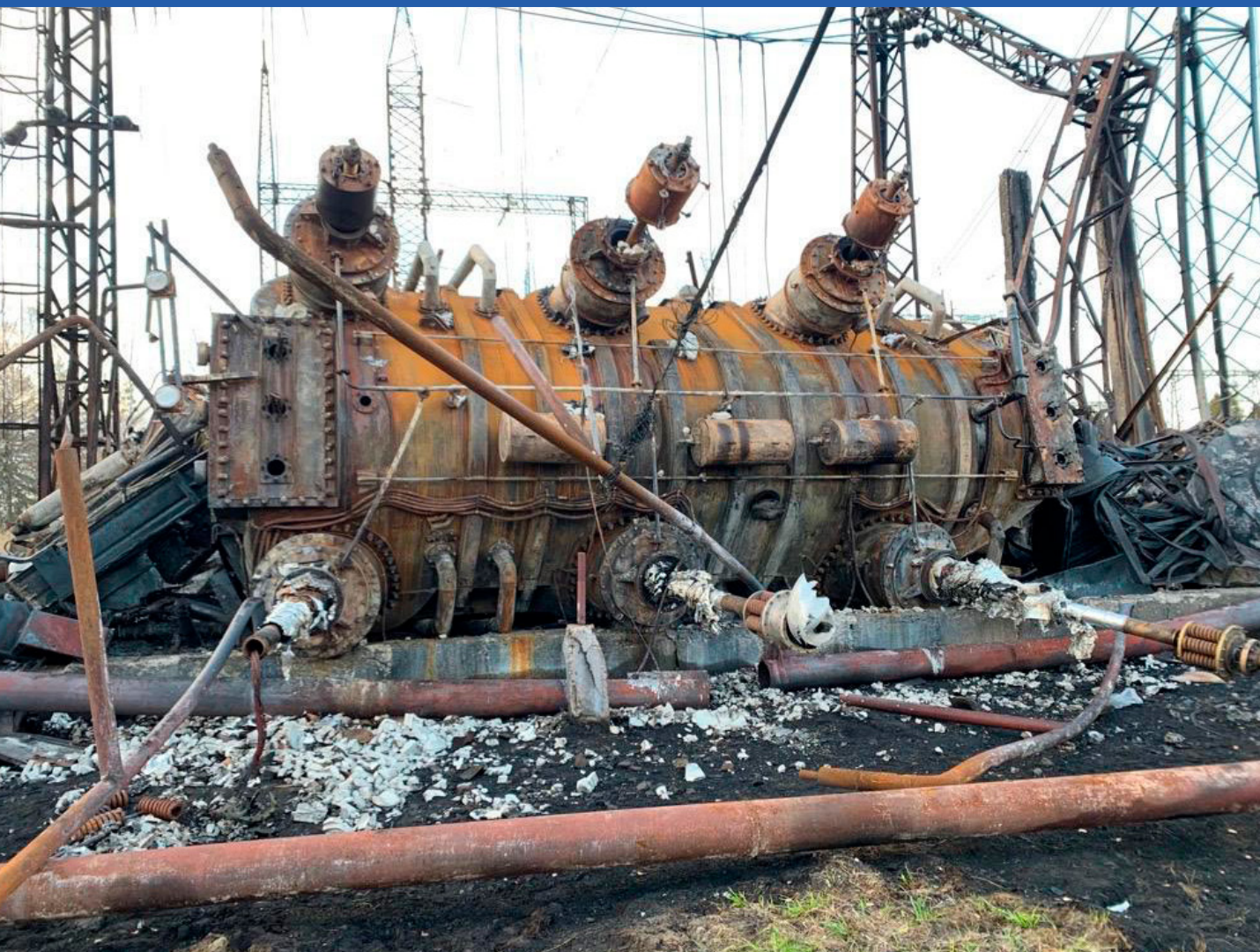
Completely destroyed 330kV 200M VA auto-transformer
